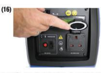
When you are ready to plug in your appliance, locate the plug socket cover at the front of the generator (15) and then lift it up to reveal the plug socket (16).
