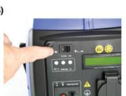
Once the engine has run for 5-20 seconds, slowly move the choke lever to the "RUN" position (move across for HY1000Si, push in for HY2000Si) (13). Before plugging in any heavy load appliances make sure the economy switch is set to the "OFF" position (14). Under normal conditions place the economy switch in the "ON" position.
