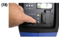
Make sure that all of the switches on your electrical devices are turned off, then insert the plug into the plug socket (17). Refer to the user manual for guidance on grounding your generator (18). We would always recommend using an earth spike. Before stopping your generator, allow to run without electrical load for 1 minute.
