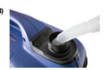
With the fuel cap removed (7), carefully pour the unleaded petrol into the fuel tank, do not overfill, leave room for expansion-25mm at top of tank (8). When the fuel tank is full, retighten the fuel cap.
